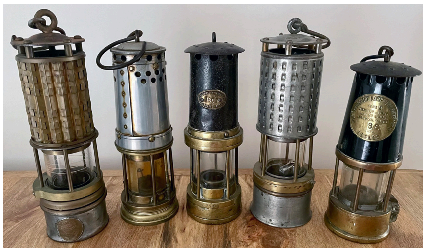
Left to right Wolf Permissible (by the US Bureau of Mines) lamp Davis Derby Boss No.3 lamp for officials, Thomas and Williams of Aberdare E. Thomas and Williams Ltd lamp, of Aberdare Makers Koehler Permissible flame safety lamp, of Marlboro Massachusetts, USA Protector Lamp and Lighting, Type SL, of Eccles, Manchester, UK
